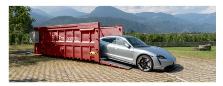
EmiControls' fire protection solutions were developed: the quarantine containers are very well suited for preventive fire protection for e-vehicles and their batteries, which need to remain under control for a certain period of time.
