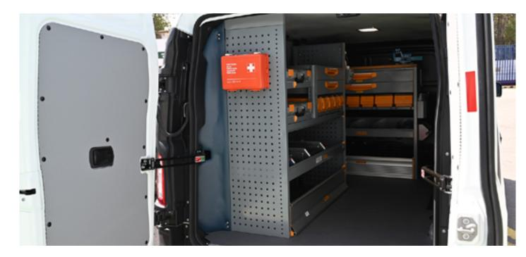
LEVC EV Mobile Service Van is designed to provide periodic maintenance and on-call service for field equipment of which cannot be brought to a workshop for repairs or maintenance. The customized van offers 24×7 on-site service support.
